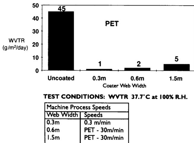
Figure 4 - WVTR Achieved on PET with SiO<sub>2</sub> Coating in Different Machines
